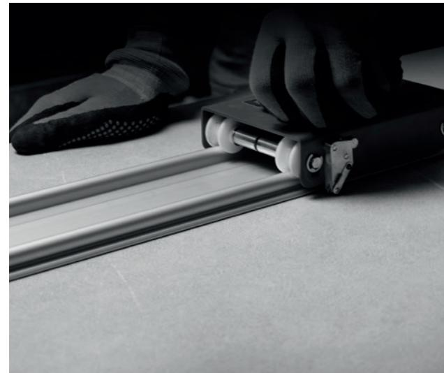
CUTTING DETAIL WITH GUIDE ON SLAB
